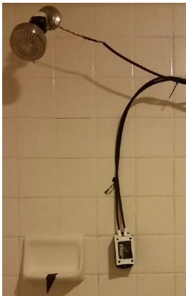
Figure 2: Flowmeter installed on showerhead
