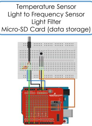
Figure 3: Schematic of the deployed sensors
