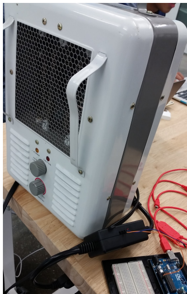
Figure 8: Fan-heater actuator with controller
