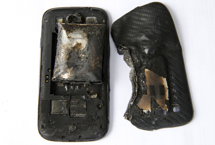
Figure 1.1: Battery Cell Failure in a Samsung Galaxy S3 Smart Phone, adopted from [1]
