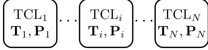
Figure 9: TCL Simulation Step. Each TCL i in the population simulates its dynamics to produce the alternative control trajectories.
